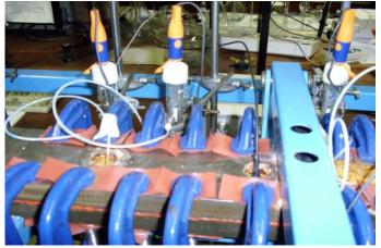
Figure 7A: Rig with the sensor probe for pH measurements
